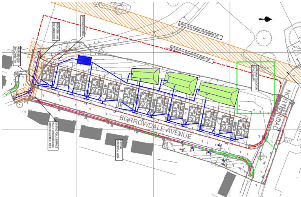
Figure One – Proposed Surface Water Drainage Scheme
